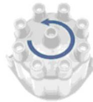
Rotor Under Cap Spins: Counter Clockwise
